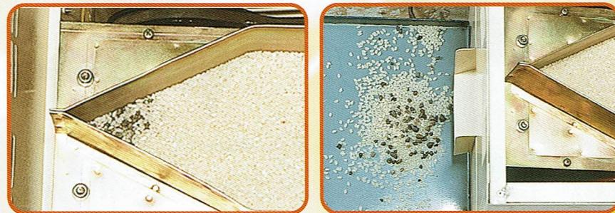
▲ None of pebbles and other matter accumulated in the triangle space (stone space) are discharged unless the stone discharge shutter is opened.
